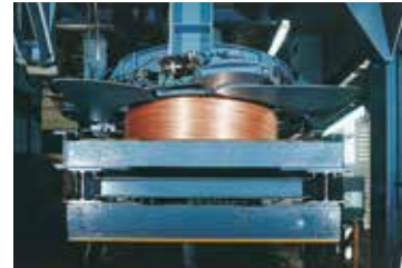
Loop laying head with ring forming chamber for wire rod coils up to 5 t
