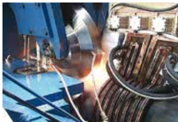
HFI tube welding
