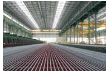
Cooling bed with high-speed delivery system (HSD®)
